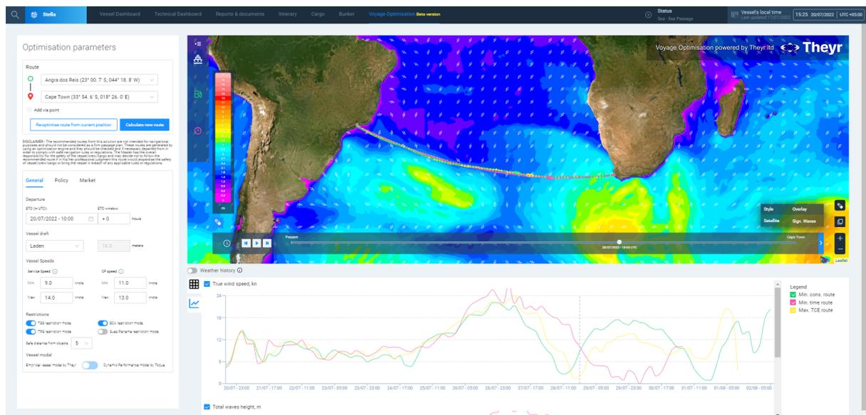
Image: Euronav FAST platform with ocean currents overlay
